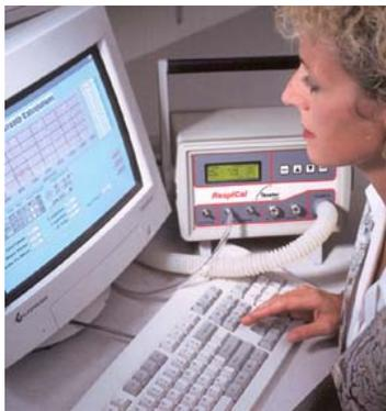
The **RespiCal** can plug into a PC above a 486 with a RS-232 socket running Windows 95 or 98 operating system.
